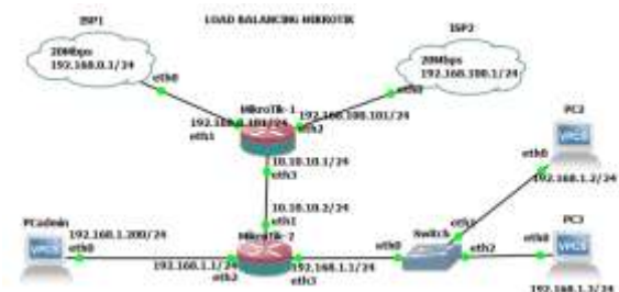
Gambar 3. Topologi load balancing Mikrotik
